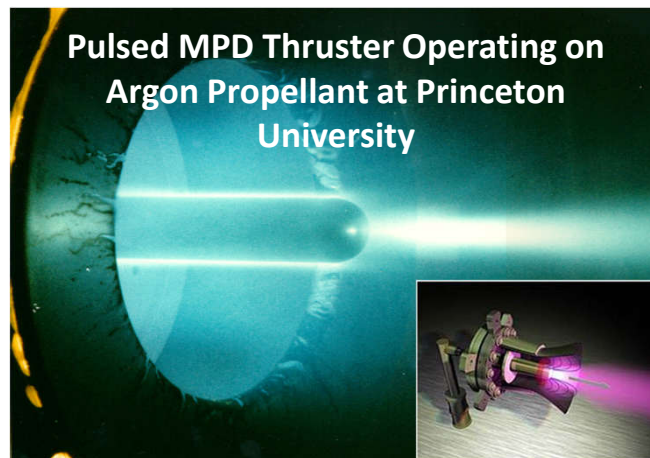
200-kilowatt MPD thruster (Credit: NASA)
