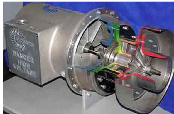
High Power Dual Brayton Test Rig at NASA Glenn Research Center (GRC)
