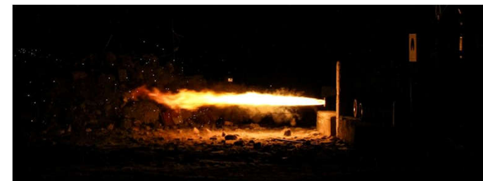
Hybrid rocket engine SL-18 (Credit: Institute SPACELINK, Trbovlje)
