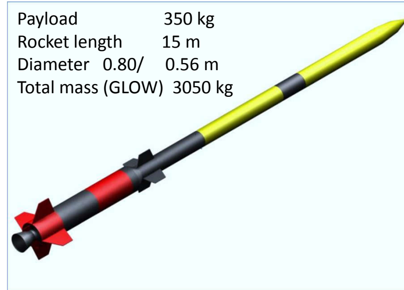
Sounding rocket and technology demonstrator VIHOR with chemical hybrid propulsion based on H 2 O 2 /HTPB propellants
