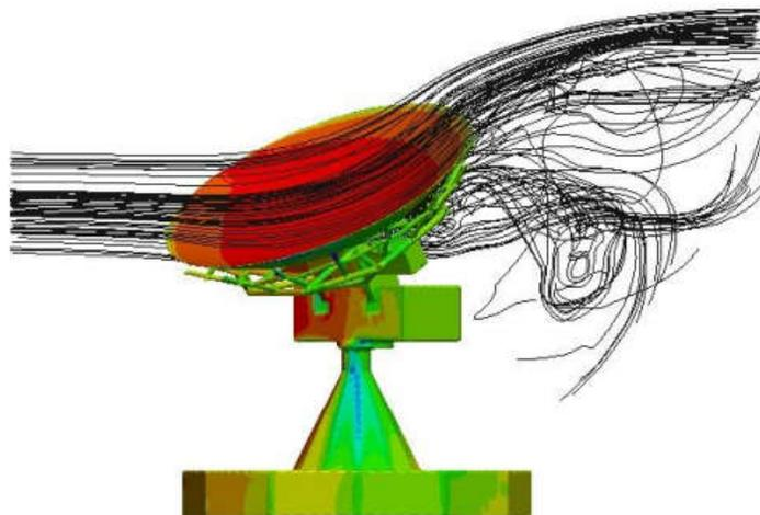
Fig. 11. The distribution of the pressure on a surface and a flow around the radio telescope. The wind direction is 45°, the elevation angle is 30°.
